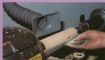
Sanding with the poseable hose fitted to the 286W makes for very effective dust clearance
