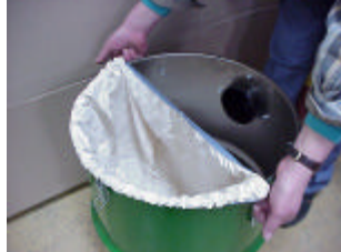
Drum filter removal
