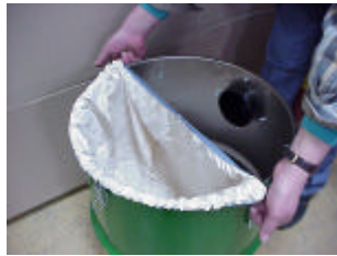
Drum filter removal
