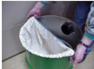
Drum filter removal
