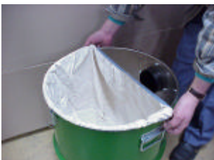
Drum Filter in place
