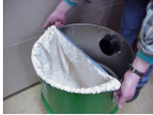
Drum filter removal
